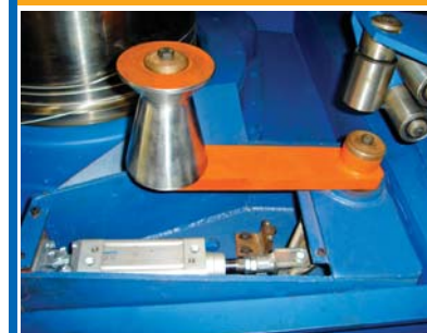
Hardened rollers- Pn. Controlled with non contact sensor
